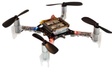
Fig. 1. The Crazyflie 2.0 nano-quadcopter. Retrieved from [26]. Copyright 2018 by Bitcraze AB.
