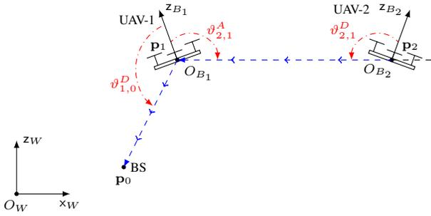
Fig. 1: Schematic of the communication relay scenario.
