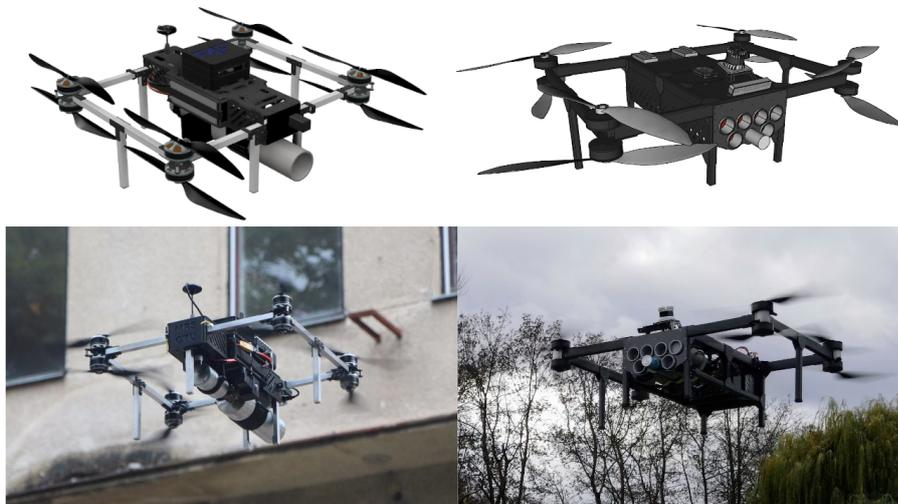
Fig. 35: DOFEC platforms (small platform left column, large platform right column) capable of autonomously launching capsules filled with a fire extinguishant into thermal sources. The top row shows CAD models of the platforms, whereas the bottom row shows them during the mission. Video: <https://youtu.be/QHpiFXzH5g>.
