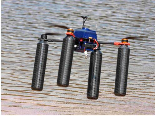
Fig. 7: Waterproof T650 platform with carbon fiber floaters.
