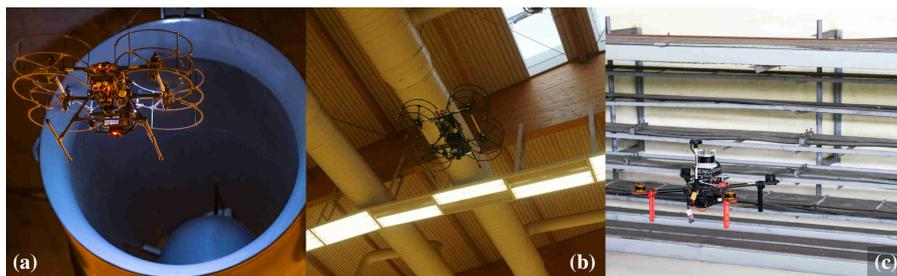
Fig. 26: Snapshots of deployment of industrial platforms (a,b) and a general research platform (c) for inspection of ventilation systems, structural degradation, and electrical infrastructure in tunnels, halls, and storage houses. Video: <https://youtu.be/60nKXamV2ds>.
