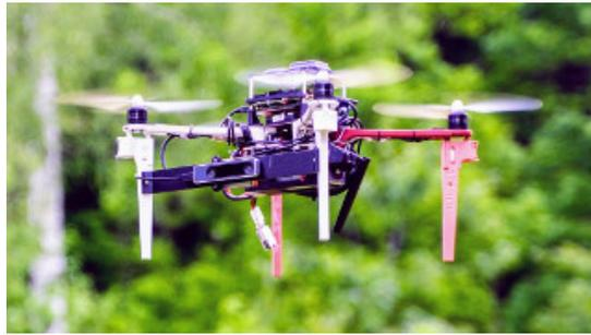
Fig. 3: DJI F450 frame used for swarming research.
