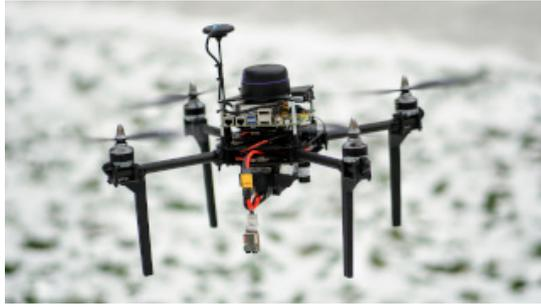
Fig. 4: Holybro X500 frame with upgraded motors.
