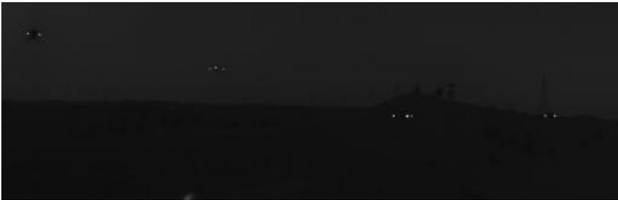
Fig. 12: View from onboard ultraviolet-sensitive cameras used in the UVDAR system. Note, the clarity of the onboard LED markers of neighboring UAVs, despite this image being captured at midday in a desert setting.
